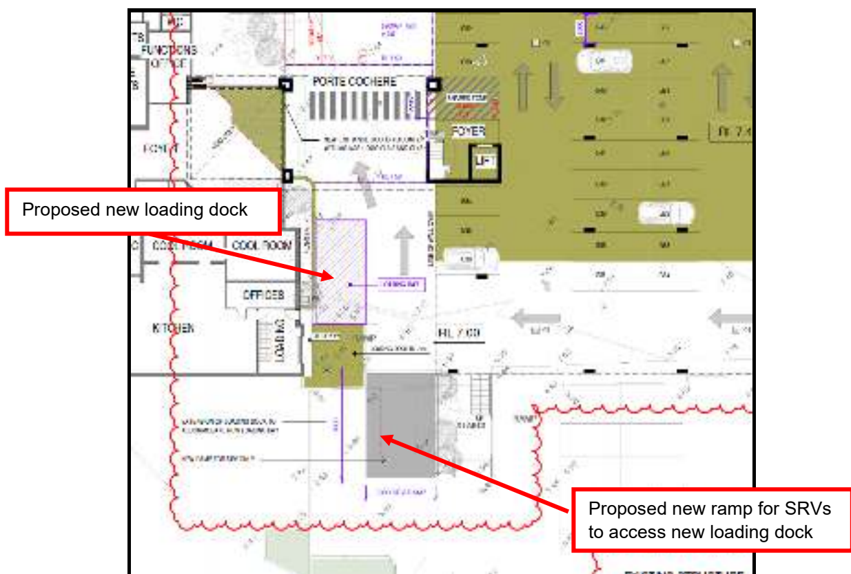
Figure 52: Proposed new loading dock on the ground floor (Source: Innovate, Rev C, July 2024)
